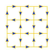
The energy for violating the constraint at two points at a distance R costs an energy  $\sigma R \Rightarrow$  confinement.
